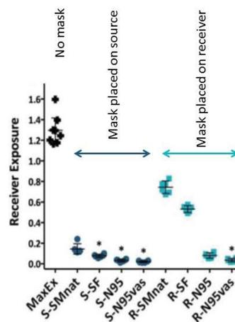
Exposure data for cough, S = Source, R=Receiver, MaxEx=Maximum Exposure, SMnat=natural fit surgical mask, SF=SecureFit Ultra fitted surgical mask, N95=3M N95 respirator, N95vas = 3M N95 respirator with a Vaseline seal.
